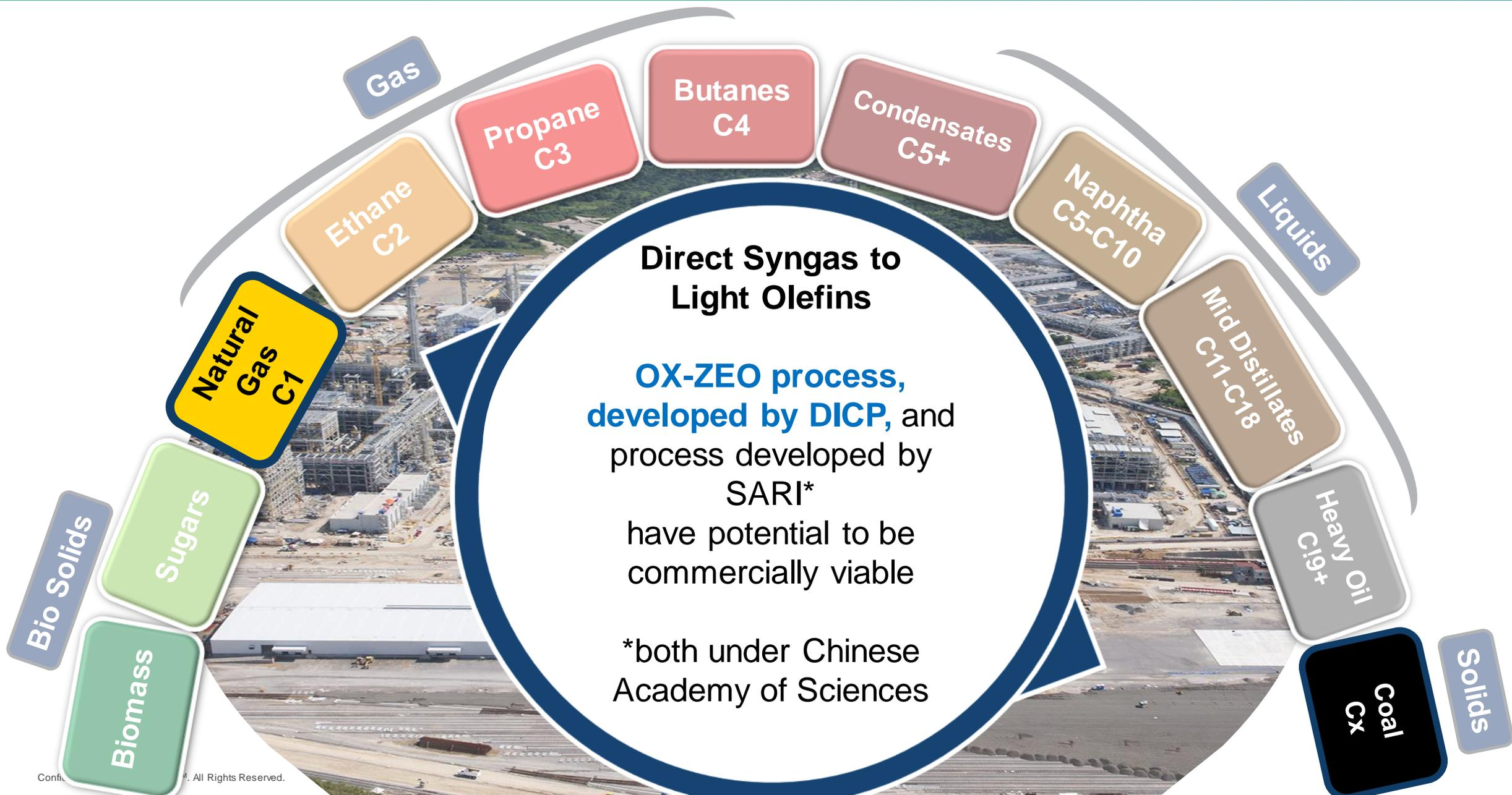
Based on an oxide of Zn/Cr metals with modified zeolite catalyst, “direct” syngas process yields high light olefins without need for a methanol intermediate
